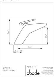
• Product mounted where: Surface • Recommended hole size: Ø 35 mm
